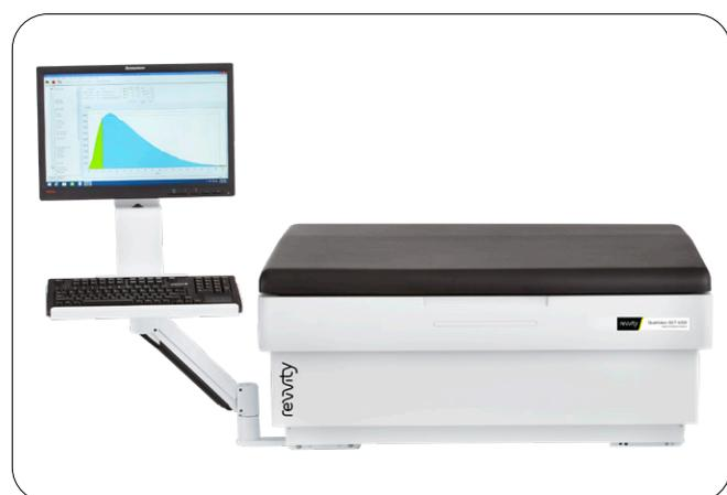
Figure 1: Quantulus GCT 6220 liquid scintillation counter.
